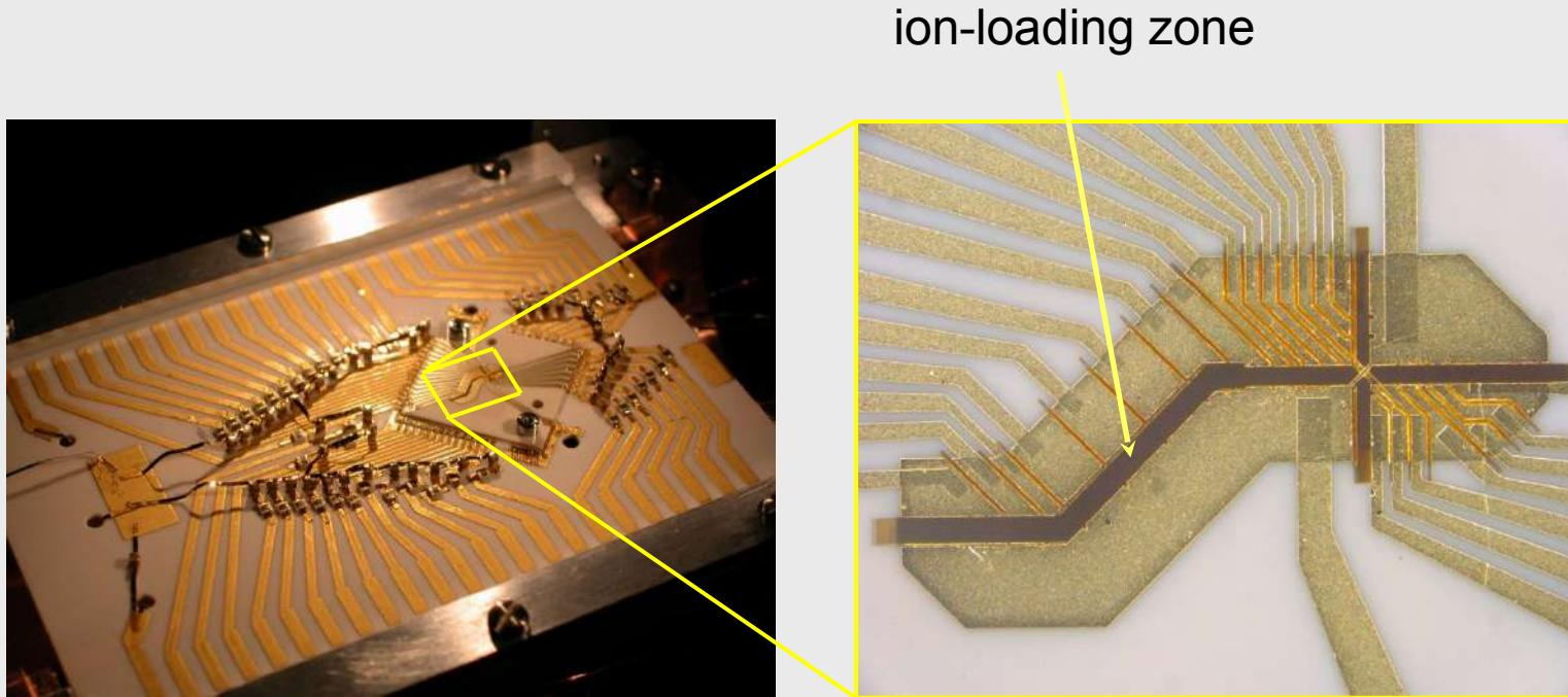
NIST, Au on  $\text{Al}_2\text{O}_3$  substrate
